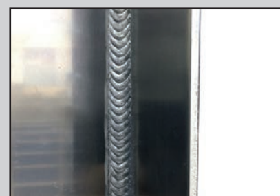
Aluminium fillet weld PF | 3.0 mm POWER.PULS (as a double pulse)
