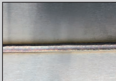
CrNi fillet weld PB | 2.0 mm POWER.PULS
