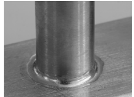
■ Circumferential weld Function: HYPER.PULS without filler material
