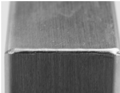
■ Corner weld Function: HYPER.PULS with filler material
