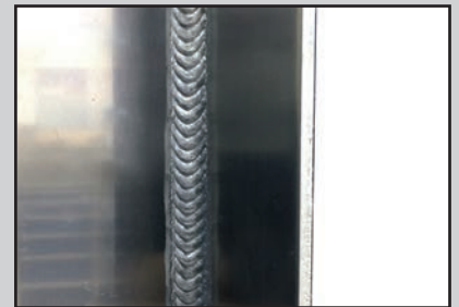
Aluminium fillet weld PF | 3.0 mm POWER.PULS (as a double pulse)
