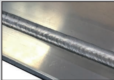
Aluminium fillet weld PB | 5.0 mm POWER.PULS
